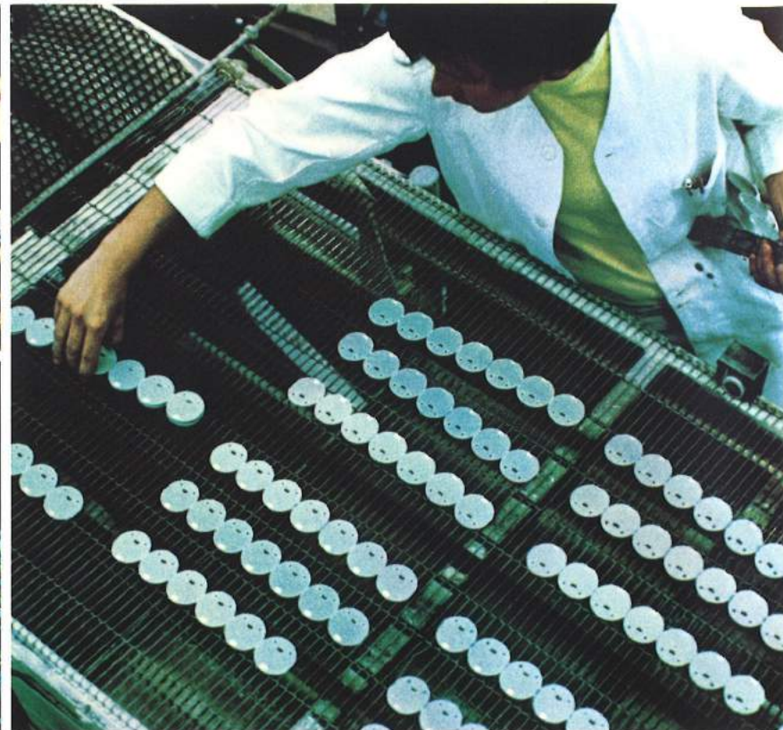
T.L. Metal stamping feed-reels and presses T.C. Glass sealing operation B.L. Curing-cycle Panelescent Nite-Lites B.C. Lamp-forming sequence R. Panelescent Nite-Lite blanks on drying rack
