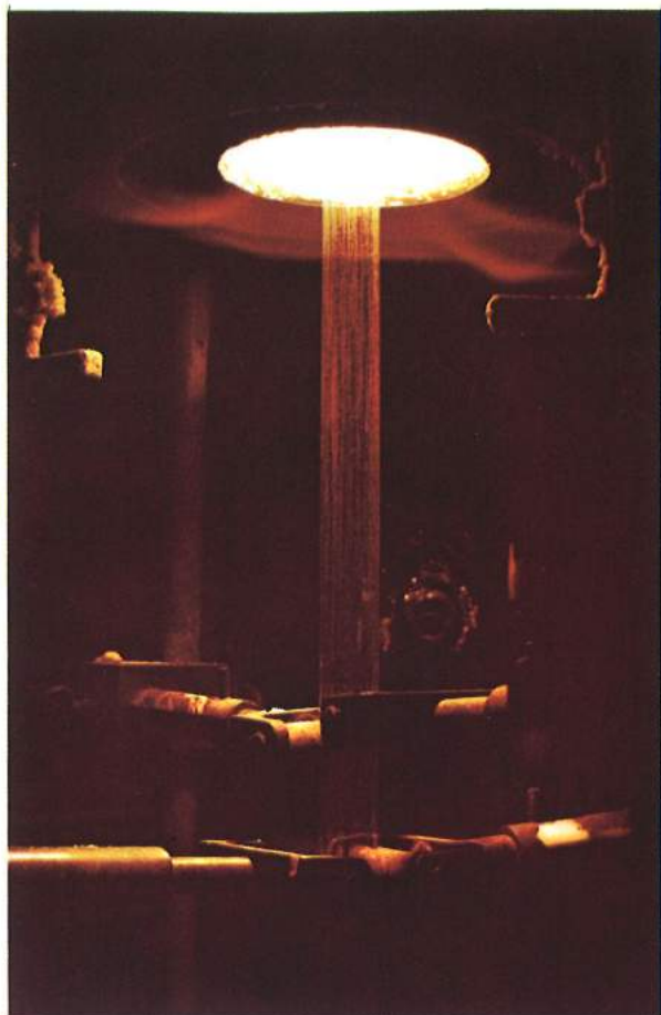
L. Drawing quartz tubing from specially designed furnace R. Detail of tube drawing clamps
